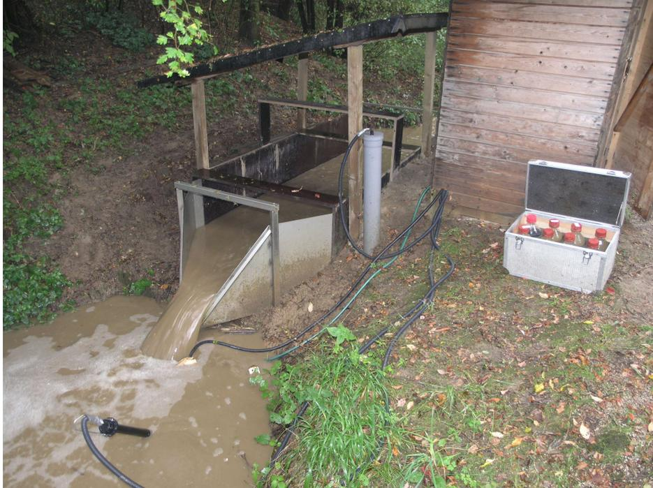
**Figure 9:** H-flume with pressure probe and additional devices at the watershed outlet.
