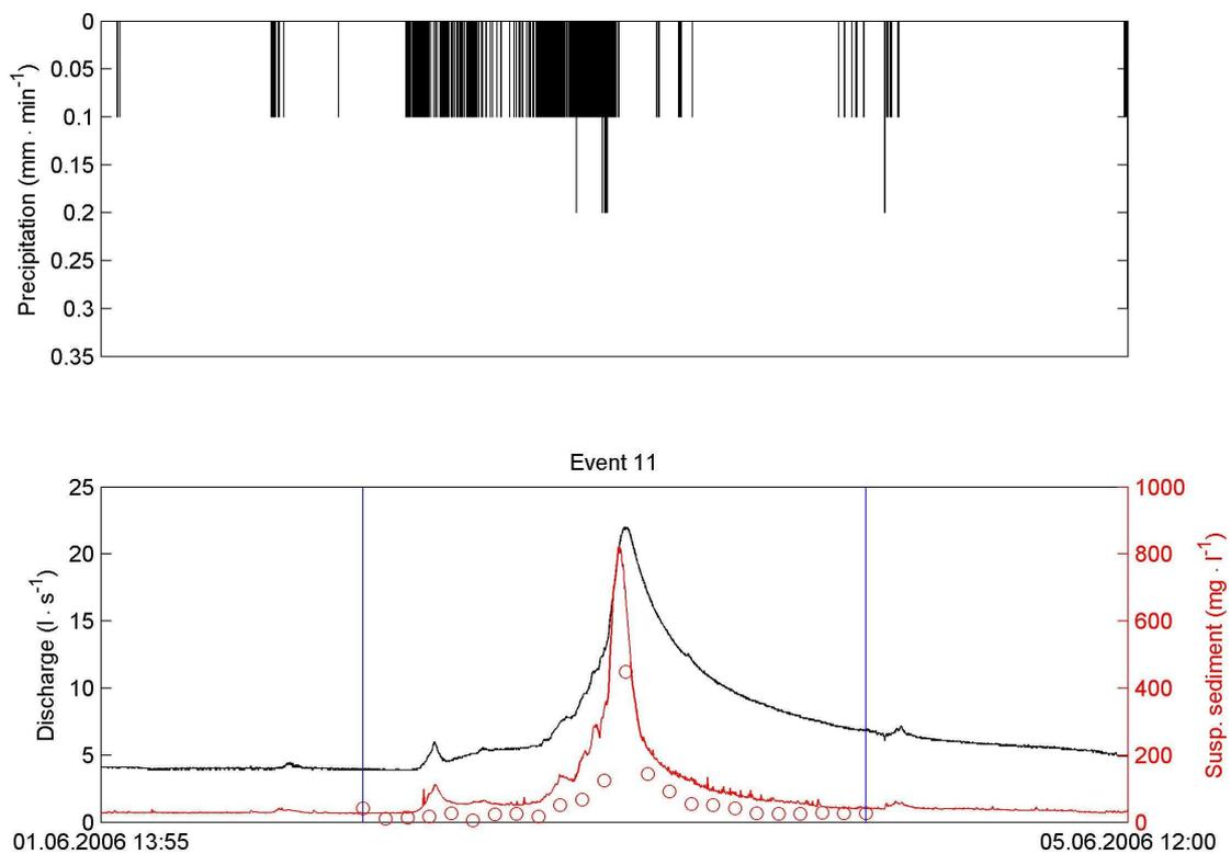
**Figure 10:** Rainfall intensity, discharge, continuous sediment concentration (Visolid, WTW) and flow proportional sediment concentrations (gravimetrically measured) for a typical event of Petzenkirchen catchment.
