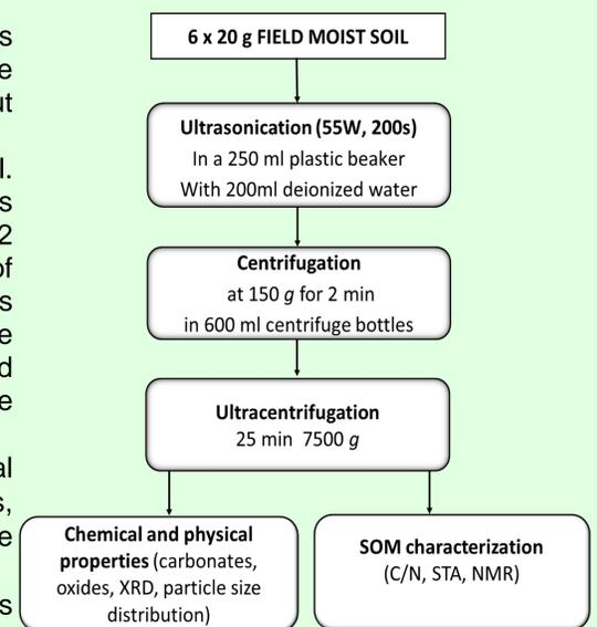
Figure 3: Protocol to gain the clay- sized particles and measurement methods
