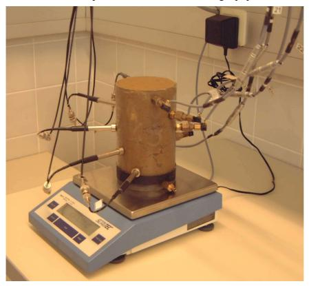
Figure 4: Equipment to determine soil unsaturated hydraulic conductivity.
